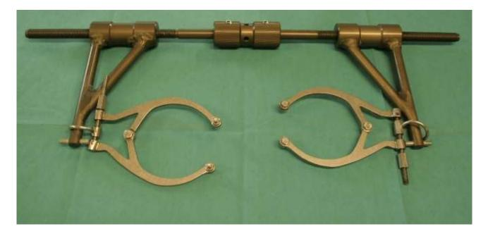
Apply two traction stirrups to the distractor as shown in the photo.
