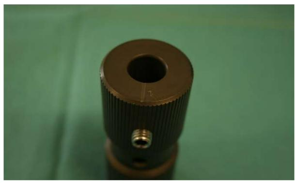
Open the locking screws on the central knob and insert the smooth part of the threaded bar and check that it is firmly screwed with the number (0,1) corresponding to that of the knob.
