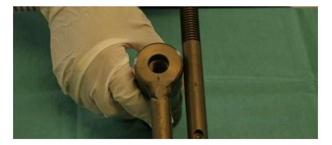
Screw the threaded bar to its bracket, referring to the number indicated. Attention: the thread of the bar marked with the number 0 is left while the thread of the bar marked with the number 1 is right.
